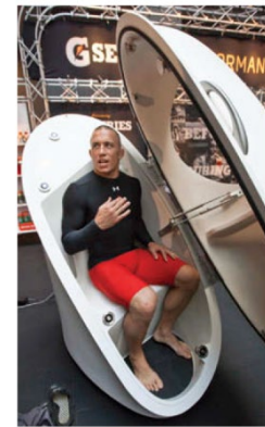
FIGURE 15.4 The Bod Pod air plethysmography device uses the air displacement technique to estimate total body volume.
